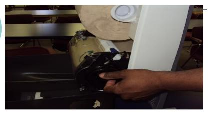
Turn the wheel on right side of dispenser counterclockwise to feed all the way through (Part 2).
